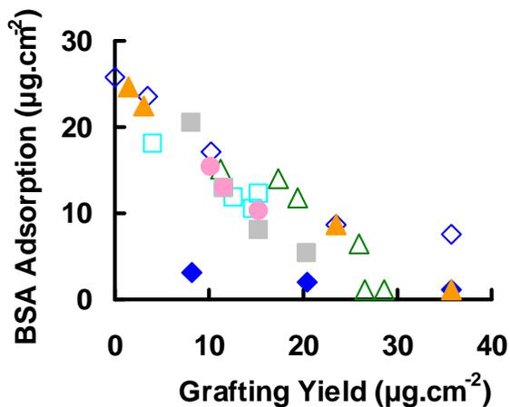
Figure 4: BSA adsorption as function of grafting yield for different reaction conditions.
