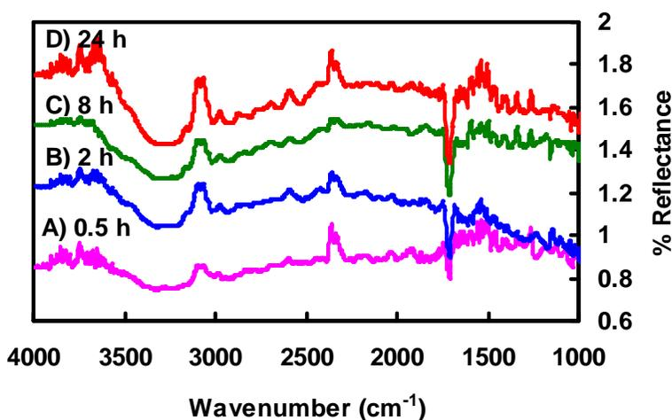
Figure 2: IR-GIR spectra for 4-hydroxybenzoic acid grafted membranes at 0.5 (A), 2 (B), 8 (C), and 24 h (D) incubation time. Reflectance is relative to unmodified membrane.
