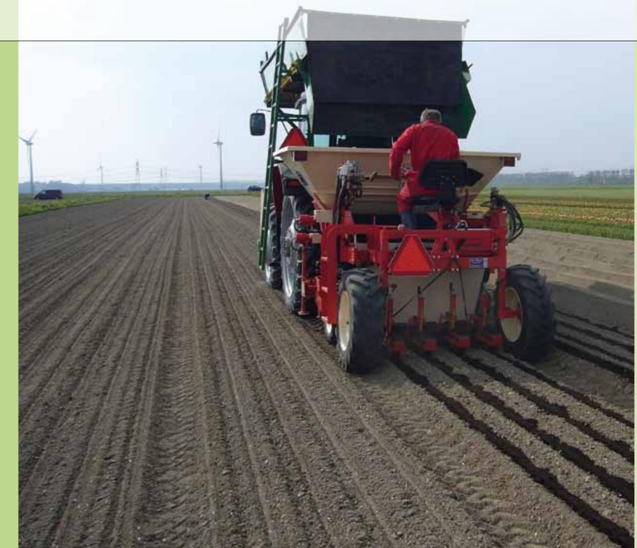
Machine which simultaneously sows and deposits a compost layer to prevent the emergence of weeds
