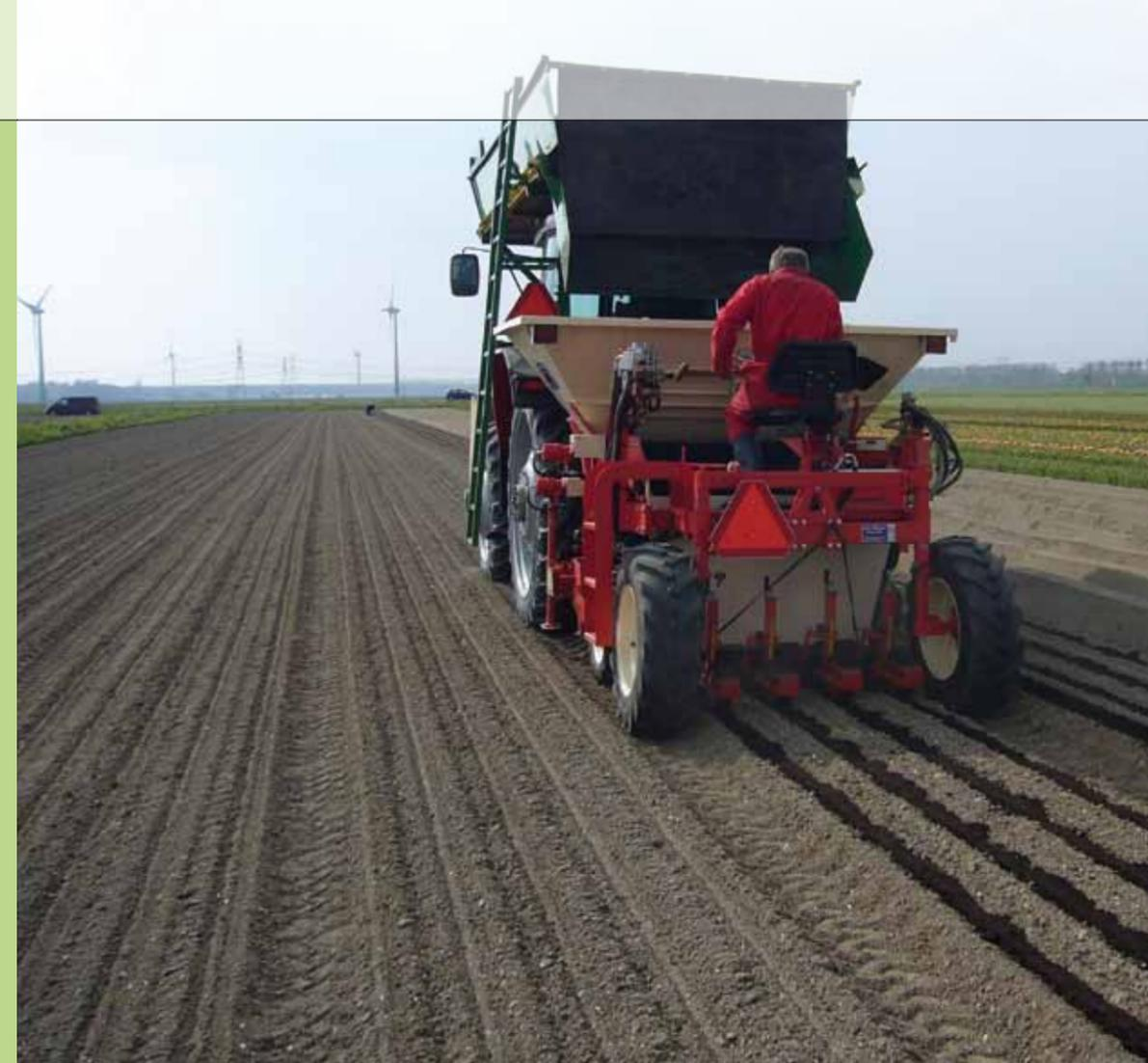
Machine which simultaneously sows and deposits a compost layer to prevent the emergence of weeds
