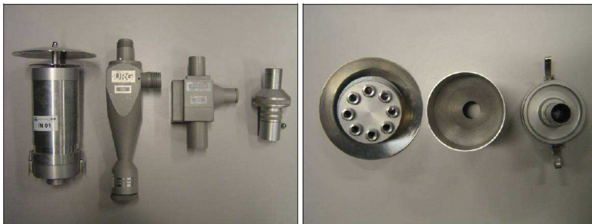
Figure 1. Sampling equipment for PM10 and PM2.5. Left (from left to right): air inlet (Ravebo Supply bv, Brielle, The Netherlands), PM10 and PM2.5 cyclones, filter holder; Right: construction of the air inlet (adapted European inlet).
