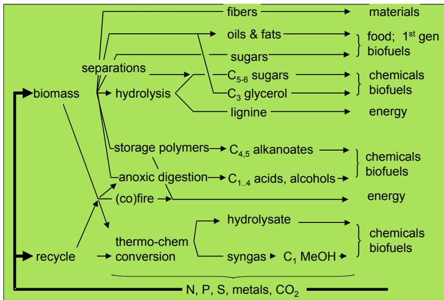
**Figure 6** Schematic and simplified overview of fractionation and conversion of biomass in desired industrial and consumer products.
