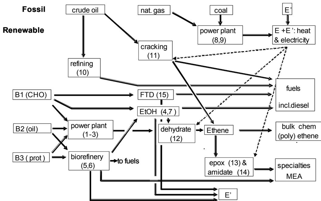
**Figure 7.** Schematic overview of the lumped processes, converting the renewable and fossil feedstocks into desired product classes.
