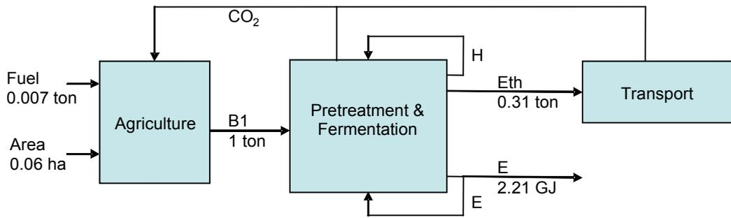
**Figure 8** Flow diagram, mass and energy balances and yield parameters of process route 4 *Pretreatment and conversion of biomass B1 to ethanol and electricity.*
