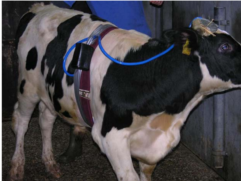
Photo 1: A pink veal calf was equipped with EEG and ECG electrodes.
