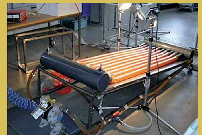
Prototype of a 100 L photobioreactor for production of H 2 by Rhodospirillum rubrum from acetate and light.
