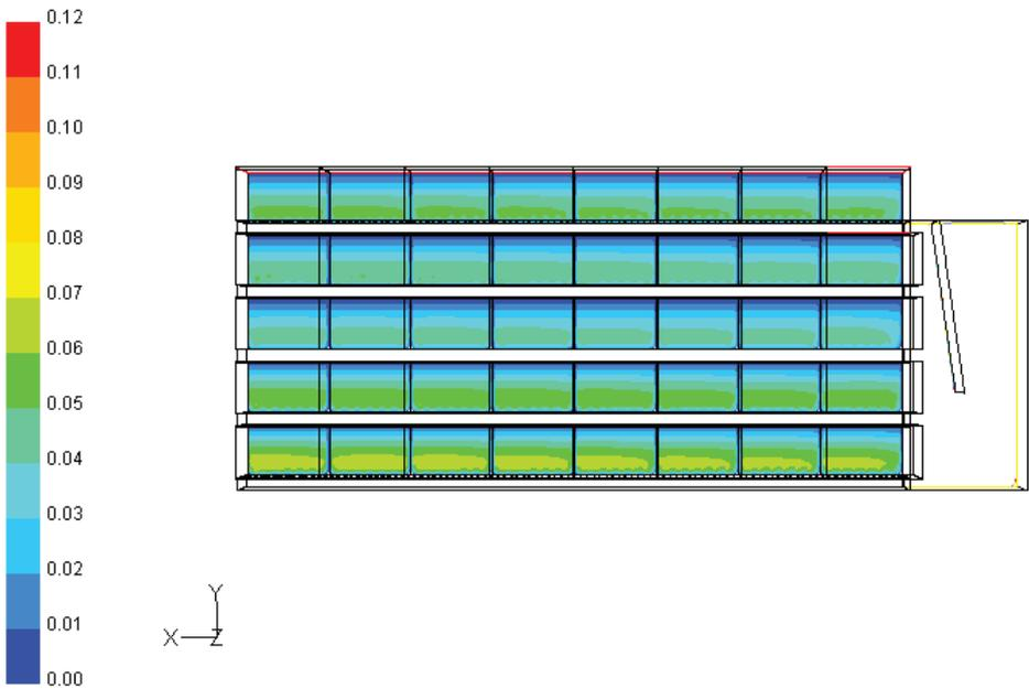
Figure 7. Air velocity magnitude of one layer storage system when the top row of boxes is covered.
