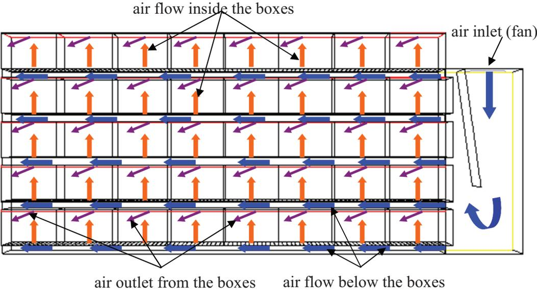
Figure 3. One layer system consists of 5 rows, 8 crates per row and an adjusted box with the ventilator.
