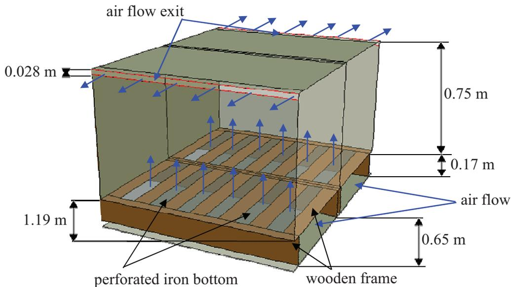
Figure 2. Typical box used for tulip bulbs storage as it was simulated in CFD model.
