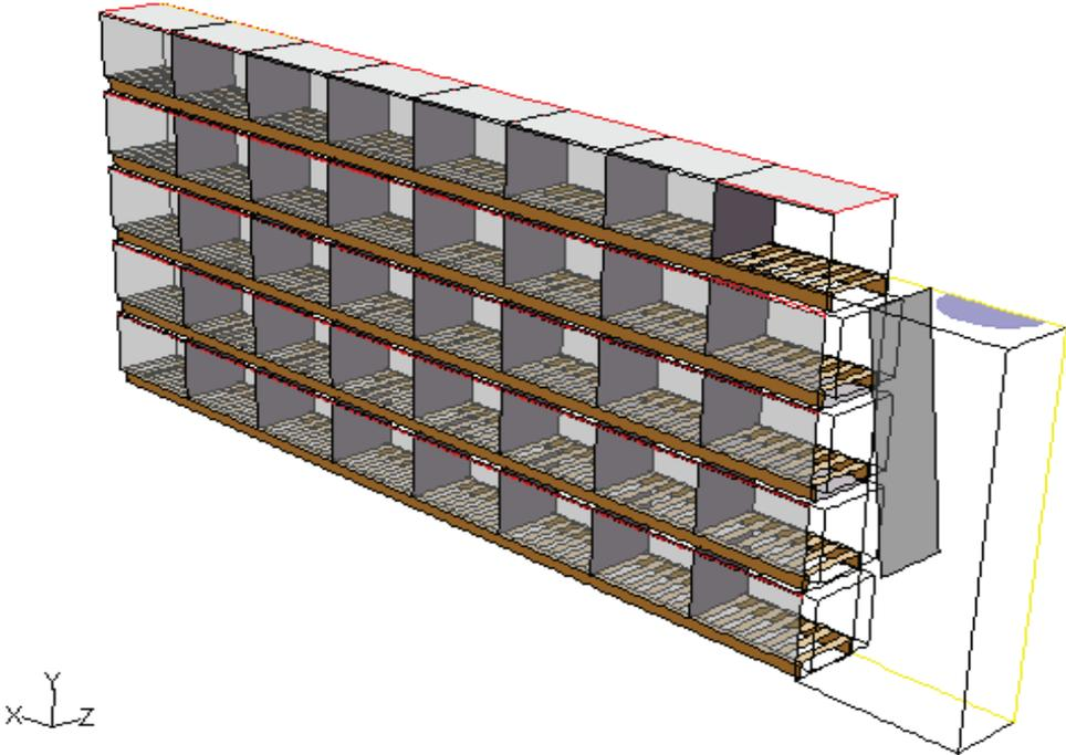
Figure 4. 3D symmetrical model of the one-layer storage system for tulip bulbs as it was designed by the geometrical processor Gambit.
