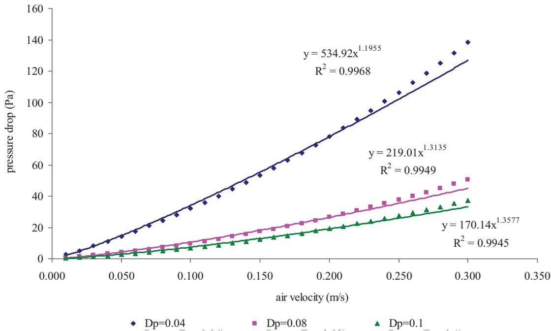
Figure 1. Pressure drop as function of superficial velocity for different tulip bulb diameters.
