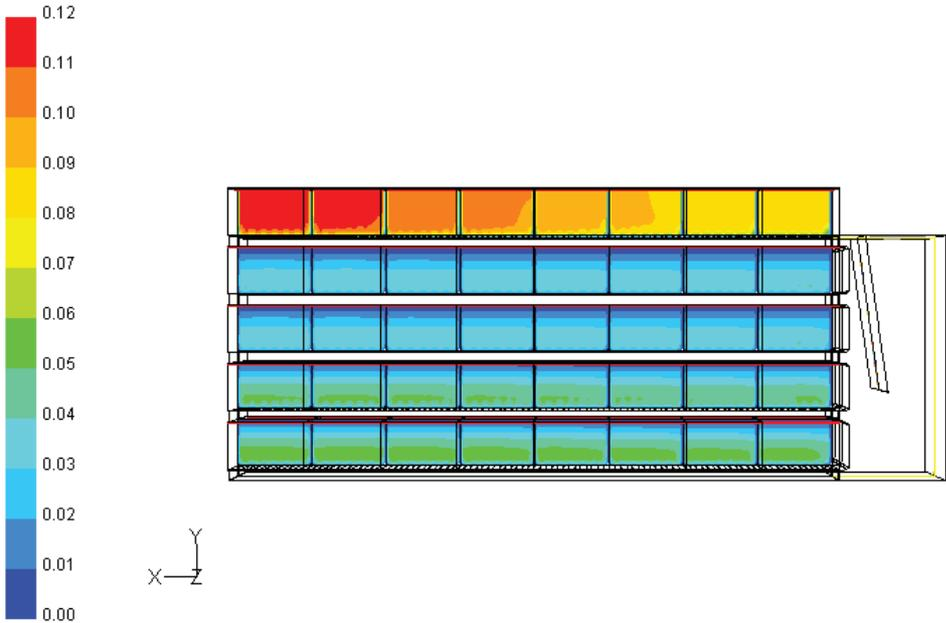
Figure 6. Air velocity magnitude of one layer storage system with smoothed sharp corners of the air flow entrance channels.
