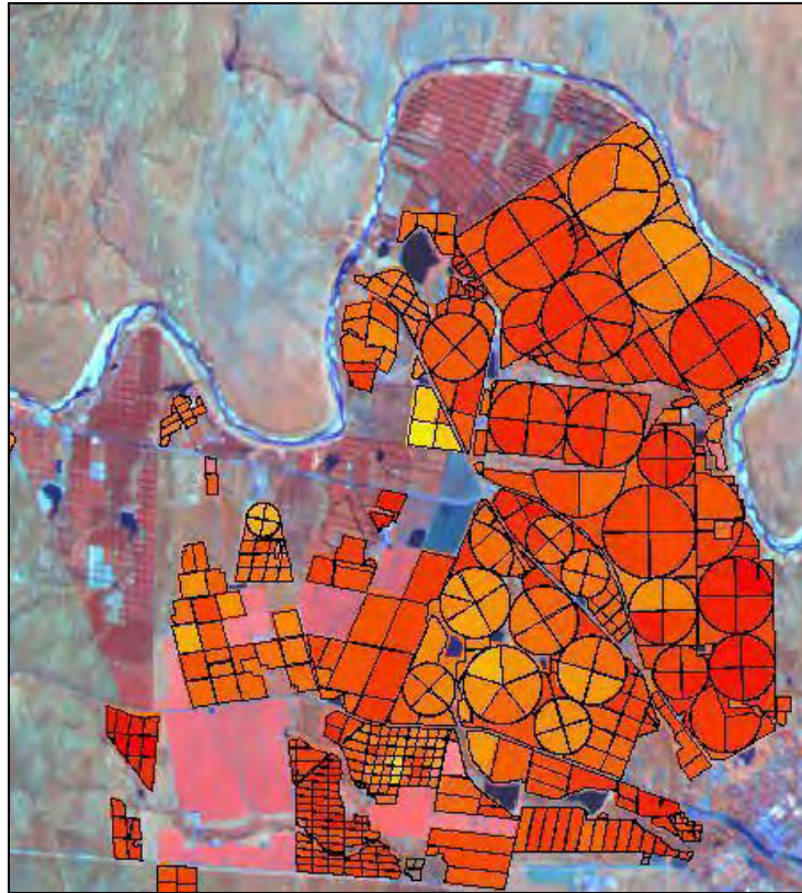
Figure 4: A subset image showing the total averaged ET of individual sugarcane fields for the 2004/2005 season. The red colours correspond to high ET values while the yellow colours correspond to low ET values.
