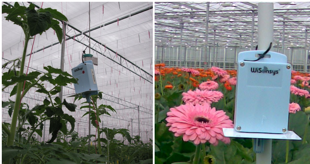
Figure 1. Wireless T-RH sensors showing the solar screen just above the sensor and mounting principles with a Pellikaan hook for tomato (left) and with a PVC-tube for gerbera (right).
