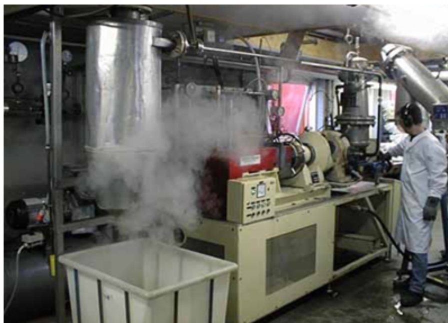
Fibre processing in a continuous pressurized 12" Andritz-Sprout-Baur refiner.
