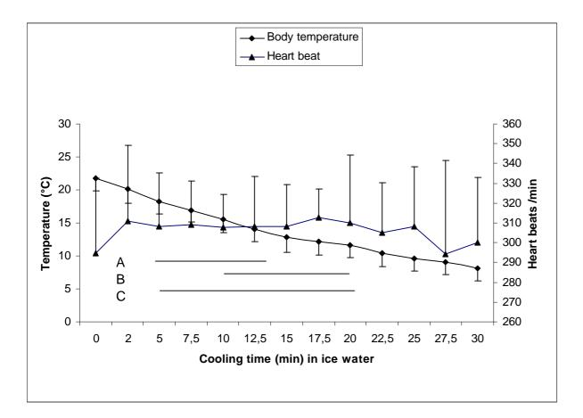
Figure 1: Live chilling of African catfish: effect on body temperature (°C) and heart rate (beats/min). The average body weight was  $1738 \pm 441$  g and the temperature of the ice water  $0.1 \pm 0.5$  °C. A= occurrence of theta and delta waves; B=low brain activity on the EEG; C= loss of pain response.
