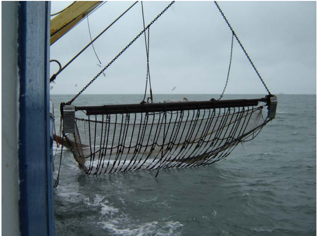
Figuur 2 Prototype 12m pulskor (november 2004)
