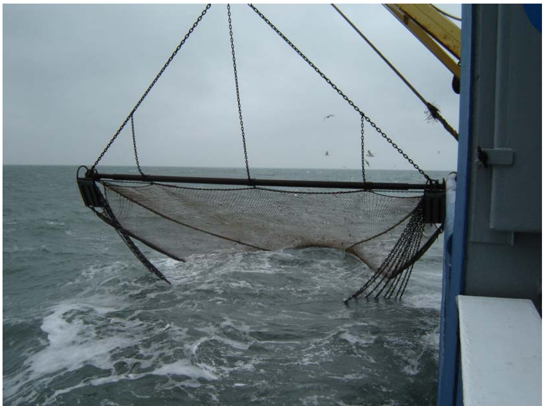
Figuur 3 Conventionele 12m boomkor (november 2004)
