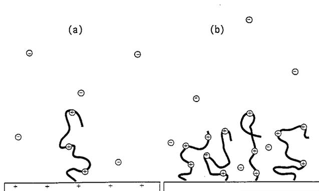
FIG. 1. A layer of polyelectrolyte chains grafted to the planar surface at low grafting density (individual chains or “mushrooms”) (a) and at high grafting density (the “brush”) (b).
