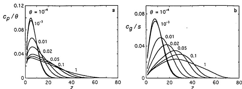
FIG. 5. The monomer density profiles (a) and the distribution of the chain end (b) for chains in a polyelectrolyte brush ( $N=200$ ,  $m=10$ ) grafted to a neutral surface, for various grafting densities. The profiles are normalized to unity. The grafting density  $1/s$  equals  $\theta/N$ ; the values of  $\theta$  are given in the plot.
