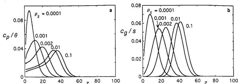
FIG. 3. The monomer density profiles (a) and the distribution of the chain end (b) for a single polyelectrolyte chain,  $N=200$ ,  $m=10$  for various surface charge densities  $\rho_s$  (shown at the corresponding curves). All profiles are normalized to unity.
