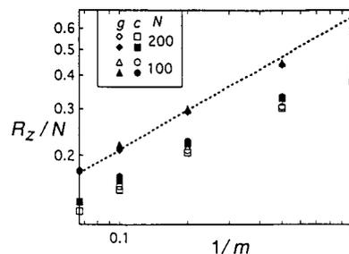
FIG. 4. The average position (open symbols) and the root-mean-square position (filled symbols) for both the end segment (diamonds, triangles) as well as for all the chain segments (squares, circles) of a single grafted polyelectrolyte as a function of the fraction of charged monomers  $m^{-1}$ , in double-logarithmic coordinates. The dashed line has a slope of  $1/2$ . The results (normalized to  $N$ ) are given for  $N=100$  and  $N=200$ ; the surface charge  $\rho_s$  is 0.1.
