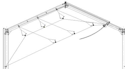
Fig. 4 Cross section of the hood with details of the suspension and steering construction of the solar cell modules, with the lowest and highest position of the modules is shown
