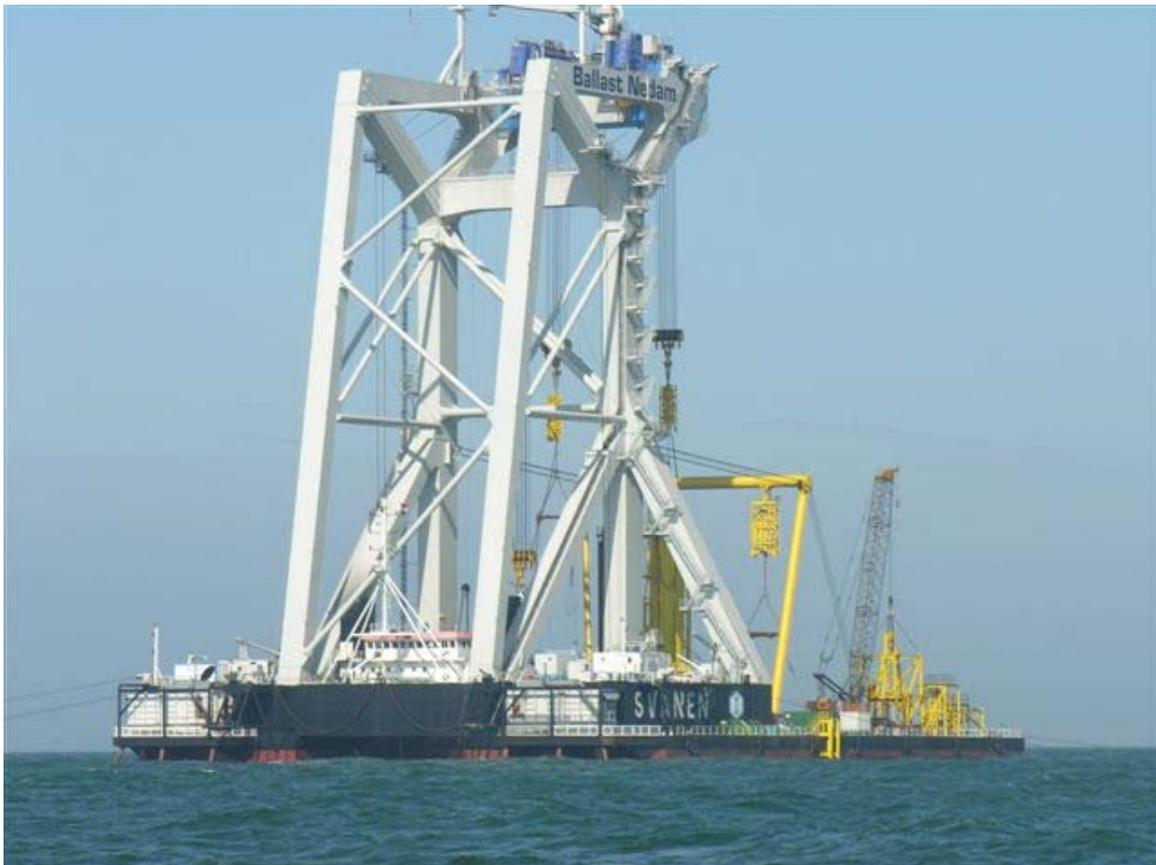
**Figure 1.** The pile driving ship "Svanen" with its superstructure rising over 100 m above sea level.
