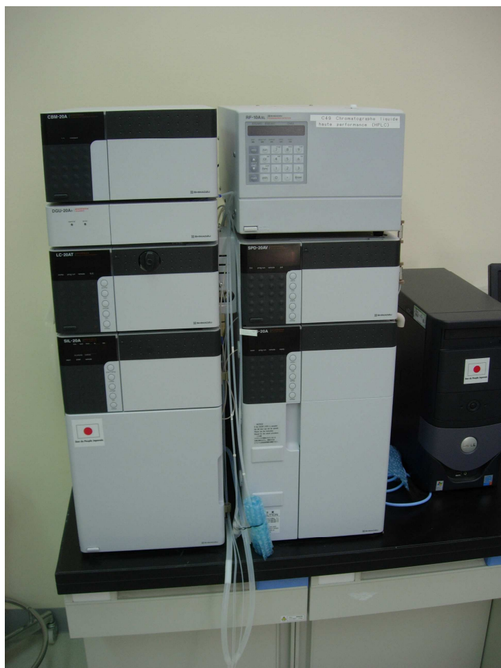
High performance liquid chromatography (HPLC) with UV and fluorescence detectors (Nouakchott)
