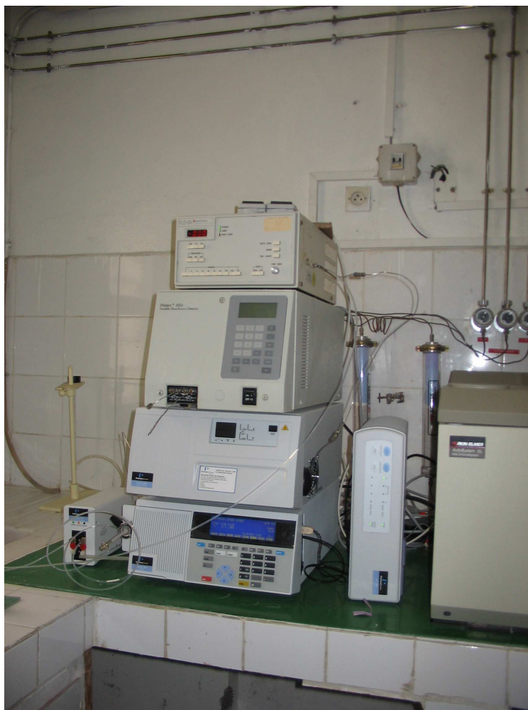
High performance liquid chromatography (HPLC) with UV detector (Nouadhibou)
