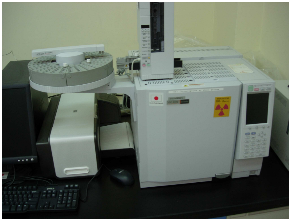
Gas chromatograph with FID and ECD detector (Nouakchott)
