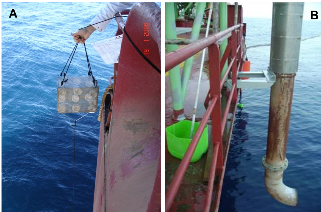
Figure 6. (A) Lowering the cage with passive samplers into sea during the first sampling campaign; (B) position of buoy with two cages during the third sampling campaign.
