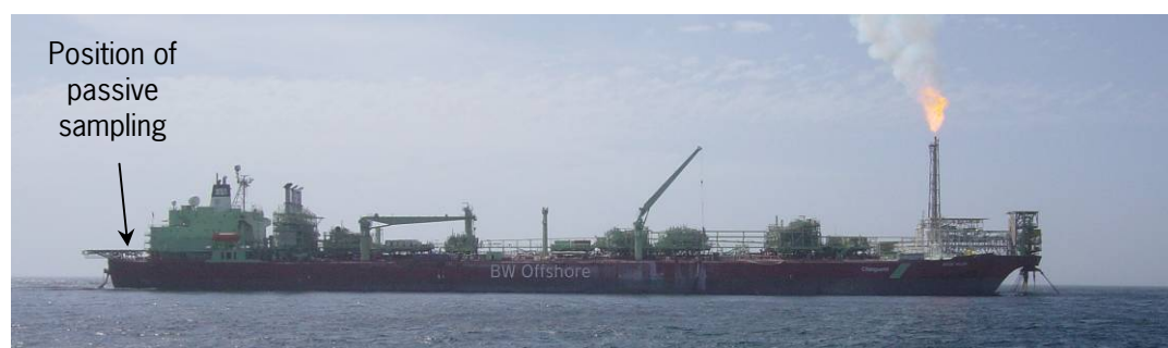
Figure 3. FPSO Berge Helene at the Chinguetti field and indication of position where passive samplers were attached.
