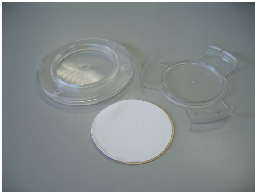
Figure 2. Polycarbonate sampler design (used in the third (post-PFW) sampling campaign).
