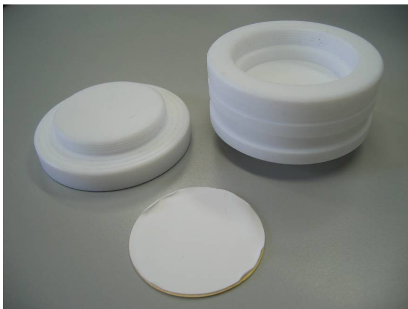
Figure 1. Teflon sampler design (used in the first and second (pre-PFW) sampling campaign).
