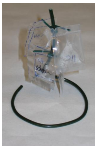
Figure 1: Wire rack for placing LDPE sachets in air stream
