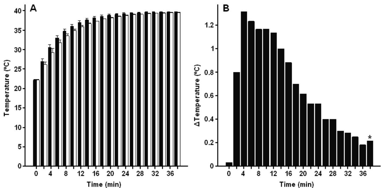
**Figure 3.** Temperature on two different positions in the hot air incubator. Temperature was measured in the left top (■) and right bottom (□). Indicated are absolute temperature (A) and  $\Delta T$  of ■ minus □ (B). Data are means  $\pm$  standard error of three(■) or two(□) replicates. \* Indicates a significant difference in temperature between the two positions in the incubator ( $P < 0.05$ ).
