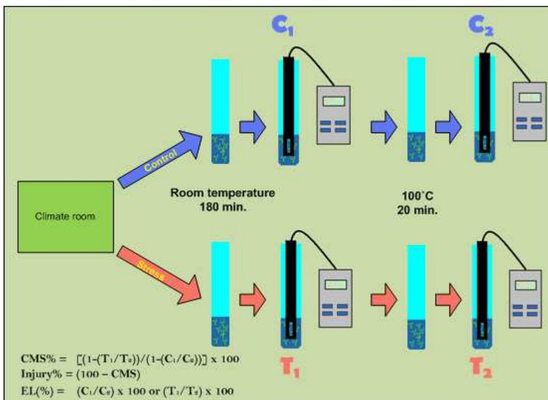
**Figure 4.** Measuring electrolyte leakage. CMS = Cell Membrane Stability; EL = Electrolyte Leakage; T = stressed samples; C = control samples; <sub>1</sub> = initial conductance reading at  $t=180$  min; <sub>2</sub> = final conductance reading after lysis of plant material.
