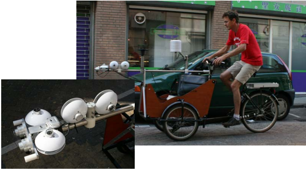
Fig. 2: Mobile biometeorological station mounted on a cargo bicycle
