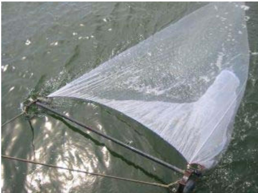
*Figure 3 2 m beam trawl net used to fish on epifauna and juvenile fish (mesh size 1 cm<sup>2</sup>).*
