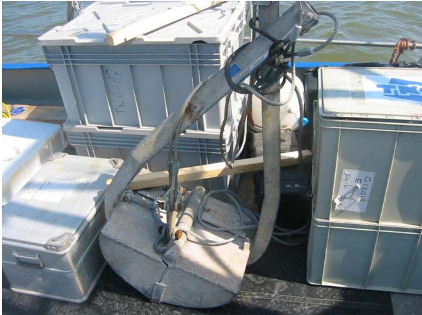
*Figure 2 Van Veen grab used to ground truth the seabed (0.1 m<sup>2</sup>).*
