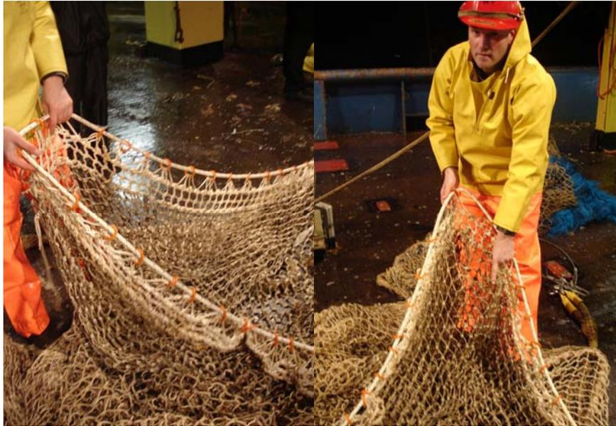
Figure 3: Benthos Release Hole (BRH1) inserted in bottom sheet of the port beam trawl, left the guider, right the escape hole (Photo P. den Hartog).
