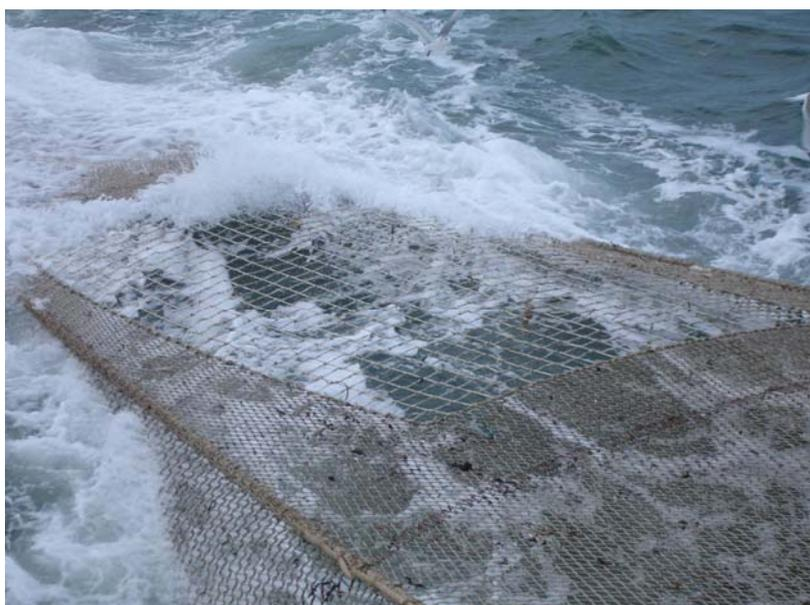
Figure 2: Square Mesh Panel (SMP26) inserted in top sheet of the port beam trawl
