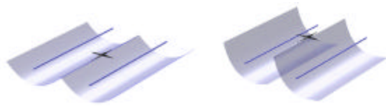
Fig. 3 Parabolic reflectors rotate in the East-West direction
