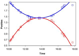
Figure 10 Both positions of the electric motors where the module will be held in the focus on August 15, 2008. R1 is the position of motor which regulate the vertical movement and R2 is the position of the motor which contribute to the horizontal movement.
