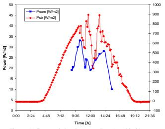
Figure 11 Generated electric power (Pnom) and incident radiation (Prad) on the location Wageningen measured on July. 31. 2008
