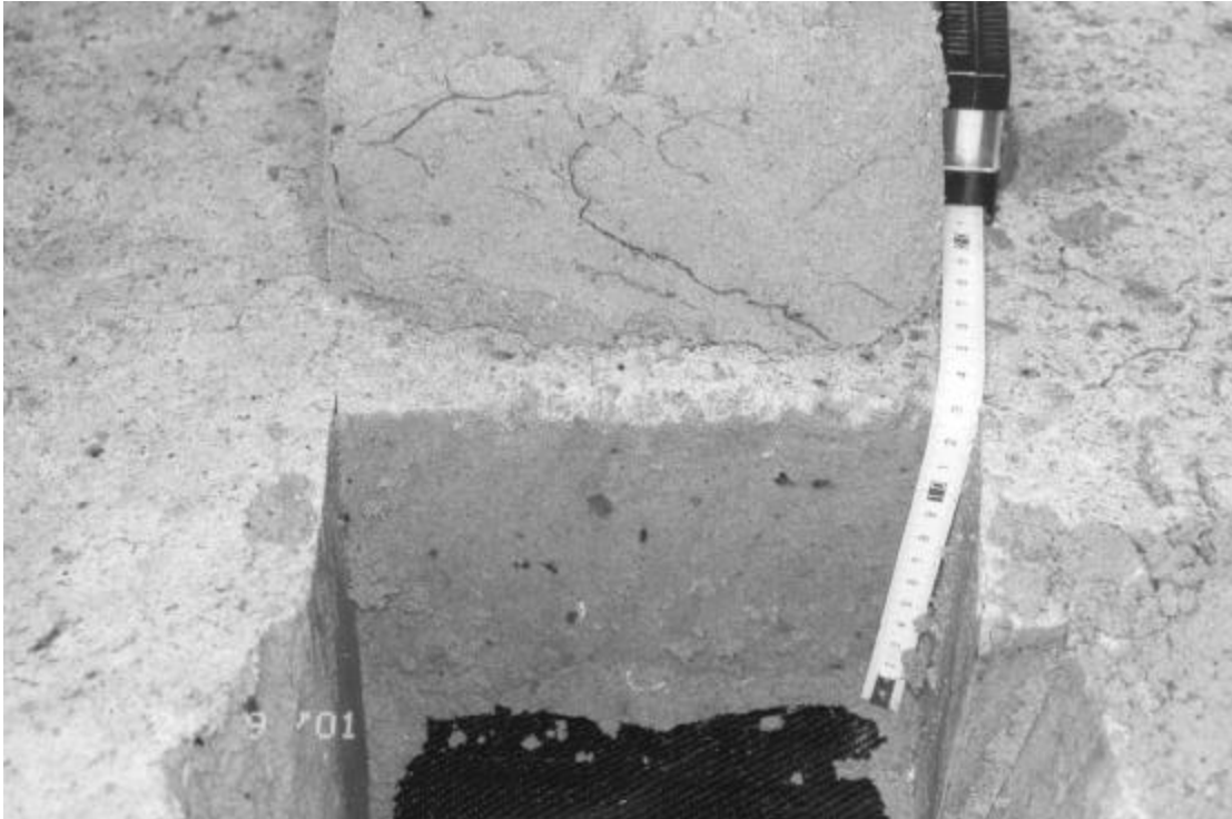
Figuur 4 Cross section of Trisoplast in the Eur 2 profile. The upper part of the picture shows Trisoplast cutted from the barrier showing plant roots at its base
