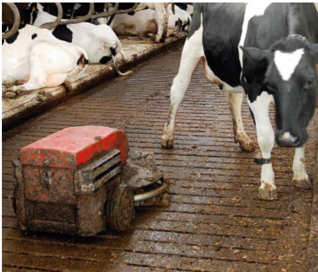
Robot route: the Lely Discovery cleaner finds its own way around the cow house
