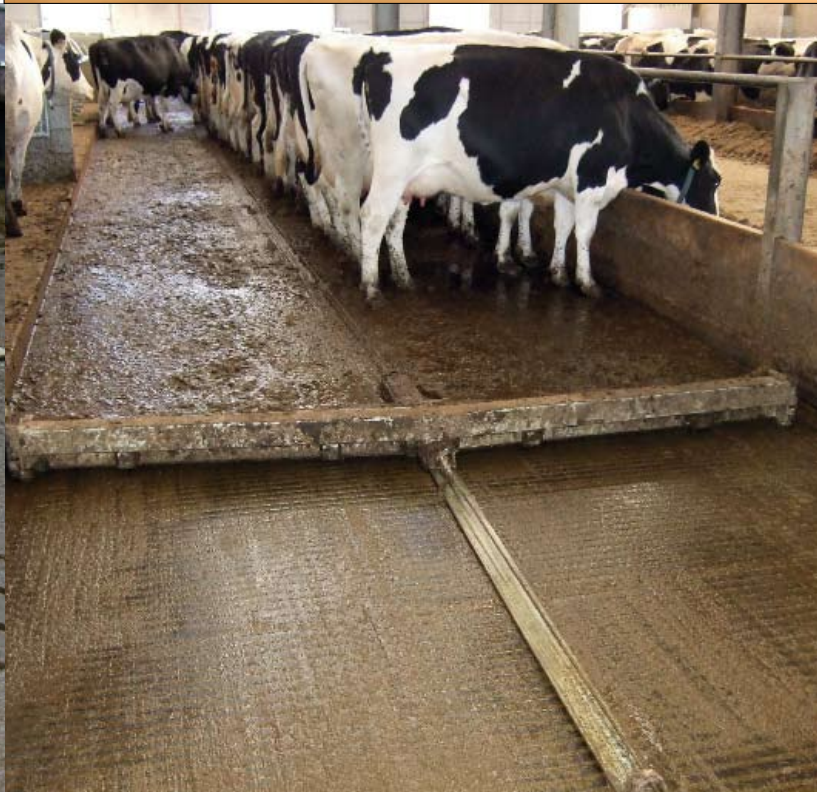
Clean concrete: scraper is designed for solid passageways
