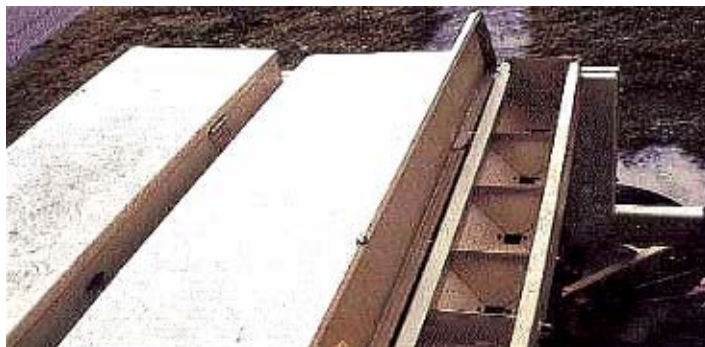
Figure 1. Truax no-till drill seed boxes: left, rear (flowable grasses), center (chaffy grasses), and right, front (flowable small seeds).
