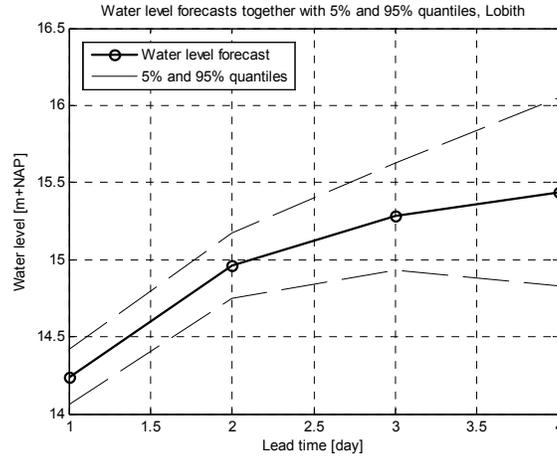
Fig. 2: Water level forecasts for four days ahead together with 5% and 95% quantiles, location Lobith, forecast model FloRIJN.
