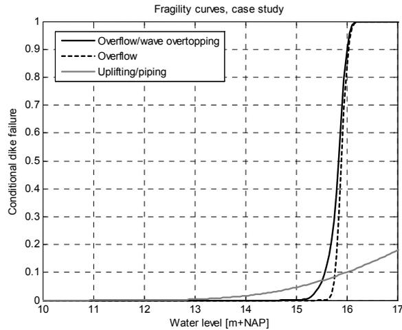
Fig. 4: Fragility curves for overflow/wave overtopping, overflow and uplifting/piping.
