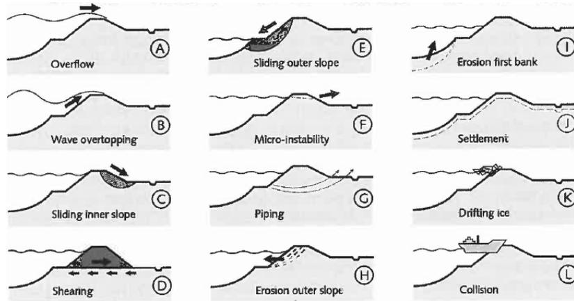
Fig. 1: Dike failure mechanisms (TAW [12]).
