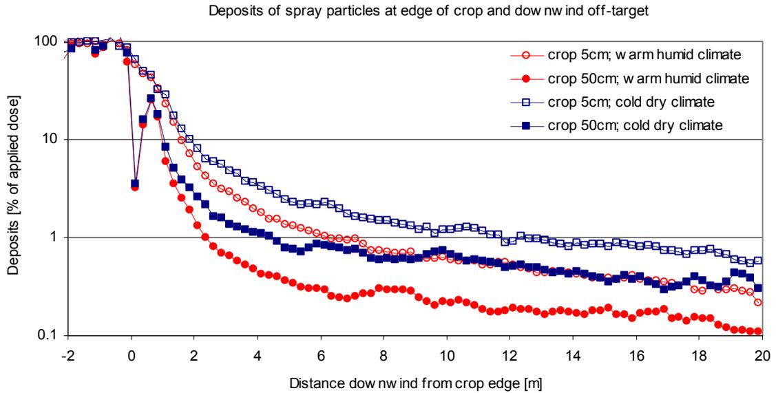
Figure 2. Ground deposits as a function of distance from the crop edge, simulated by the IDEFICS model.
