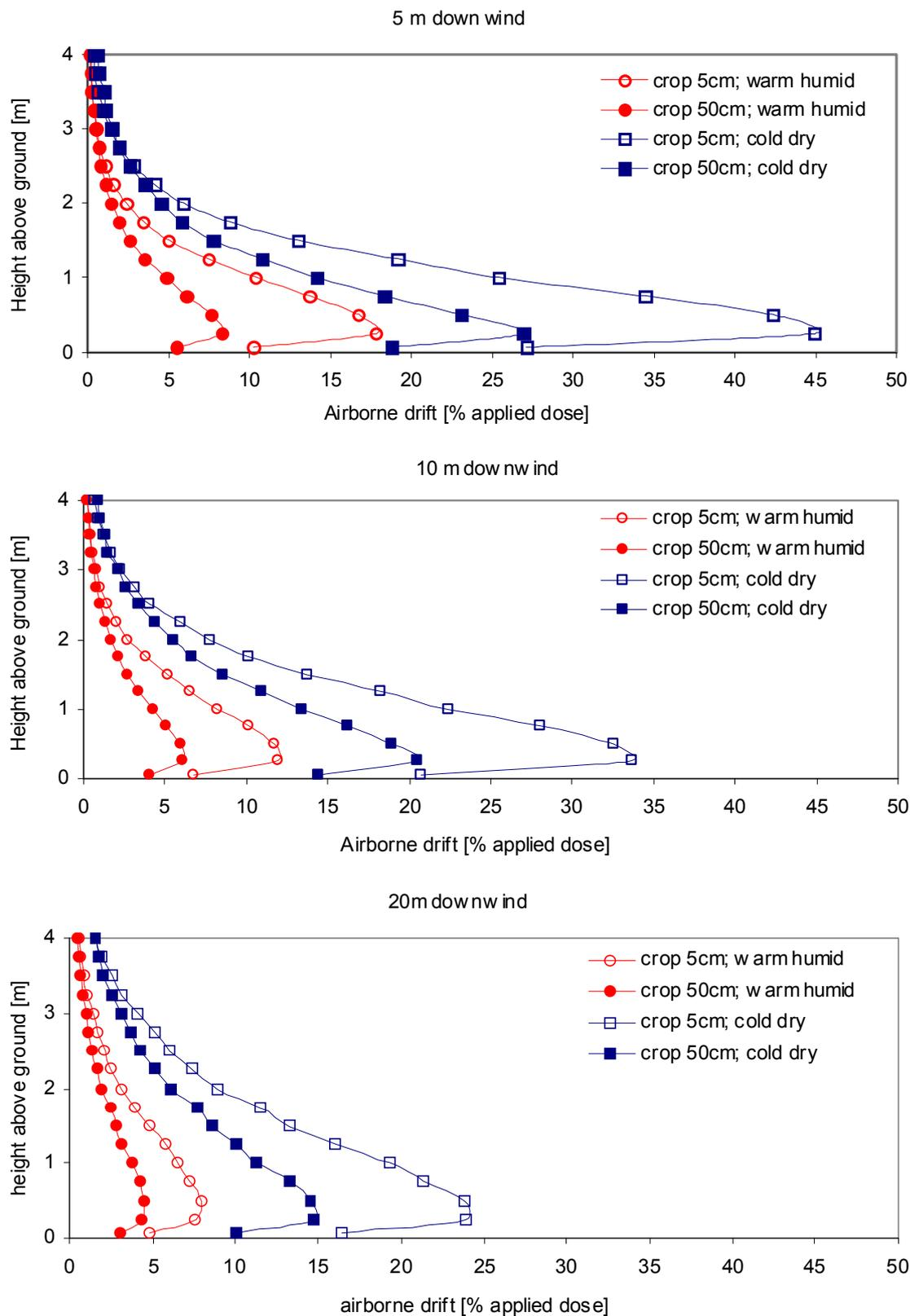
Figure 3. Vertical distribution of airborne spray downwind at 5 m, 10 m and 20 m from the crop edge, simulated by the IDEFICS model.
