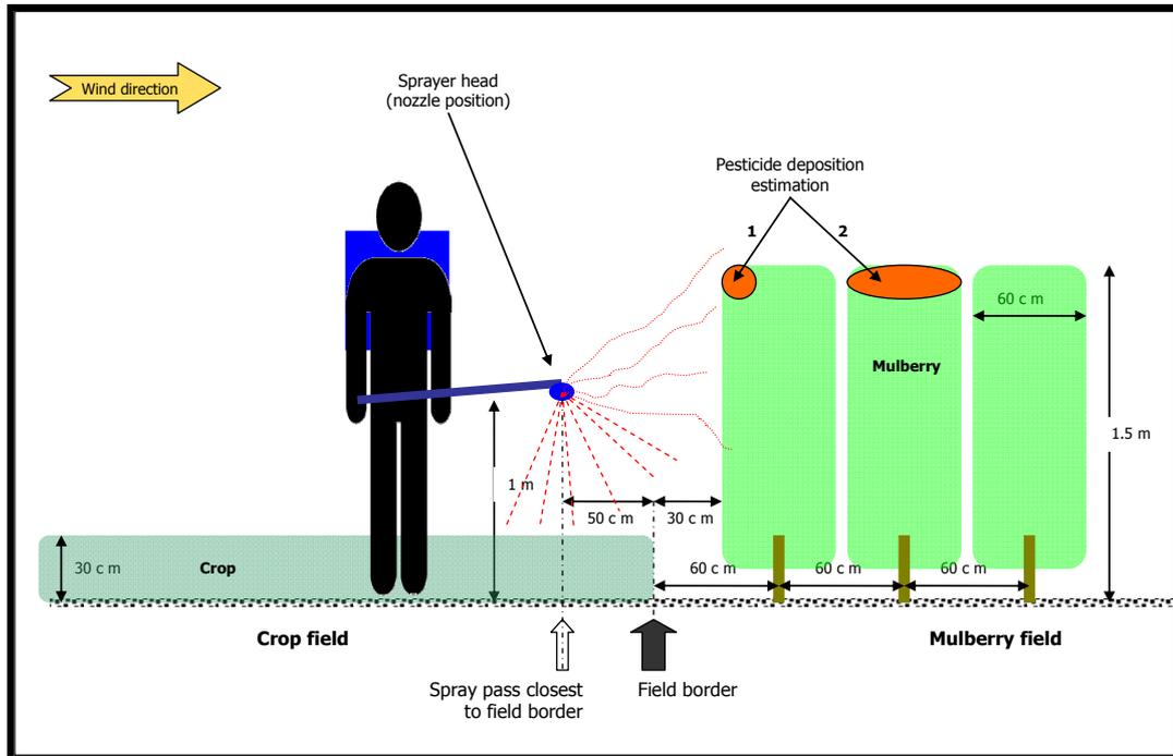
Figure 4. Reference situation for estimating the spray drift on mulberry trees.
