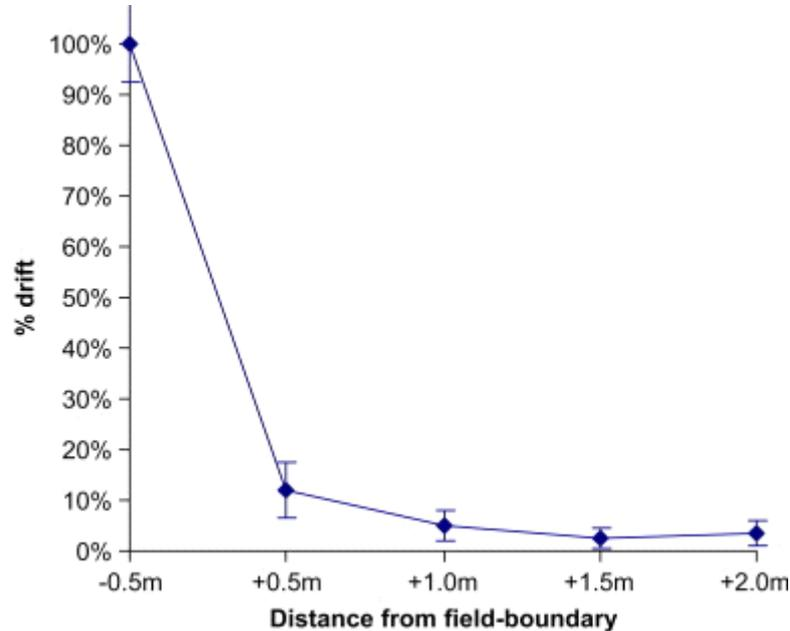
Figure 6. Pesticide deposition from knapsack sprayers in rice in the Philippines, expressed as the percentage of the applied dosage per unit area, average from 17 farmers (source: Snelder *et al.*, 2008). Error bars represent the standard deviation of the mean.
