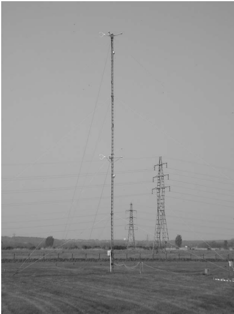
Figure 1. Experimental site with tower for radiation divergence observations in Wageningen, Netherlands (view is in western direction). Photo by Oscar Hartogensis.
