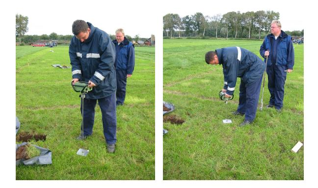
Figure 8. Measuring penetration resistance in the field using a penetrologger. A cone (top angle  $60^{\circ}$ ) with a surface area of 1 cm<sup>2</sup> is placed at the end of the rod (about 1 m long). The rod is pushed into the soil with a speed of about 2 cm/s. Speed and depth are measured using a sensor that sends a signal to the reflector plate resting on the soil surface.
