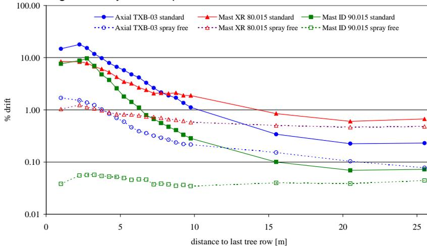
**Figure 1.** Spray drift deposition on soil surface next to a nursery tree field when spraying with a standard axial fan sprayer equipped with hollow cone nozzles (TXB-03) and the mast sprayer equipped with standard flat fan (XR80015) and low-drift venturi flat fan (ID90015) nozzles in a standard situation and with a 5 m spray-free buffer zone
