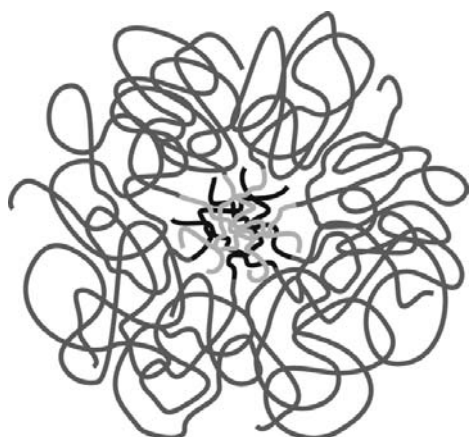
Fig. 1. Schematic representation of a complex coacervate core micelle (C3M) consisting of two diblock copolymers. The cationic (light grey) and anionic (black) polyelectrolyte blocks of the copolymers reside in the micellar core, while the neutral, water-soluble segments (dark grey) form the micellar corona.
