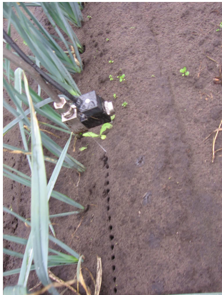
Figure 1. Injecting pesticides or fertilizer directly into the rootzone at 125 bars and in Pulstec mode
