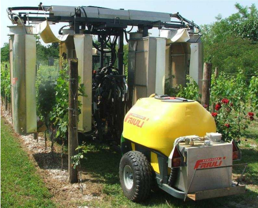
Figure 1 . The prototype tunnel sprayer.
