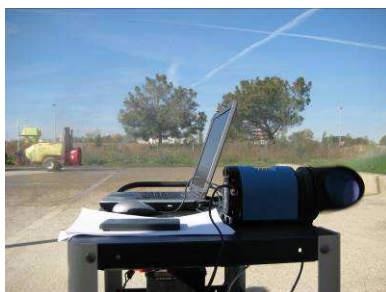
Figure 1. Spray drift measurement with the LD-LRS 1000 sensor
