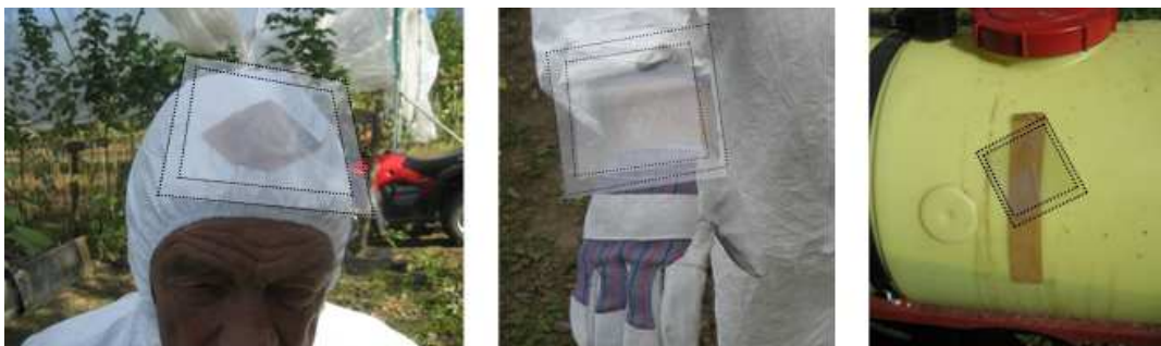
Figure 1. Passive samplers, size 10 x 10 cm 2 fixed on a 12 x12 cm 2 layer. Dotted lines show the edges of the samplers and supporting layers. Sprayer tank pulled by the ATV for raspberry on the picture to the right. An inner tape was used to fix the bottom layer.
