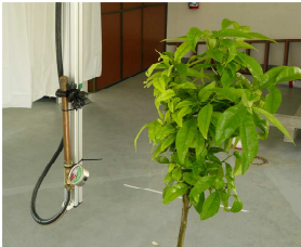
Figure 1. Spraying of infested seedling with the simulate spray system.
