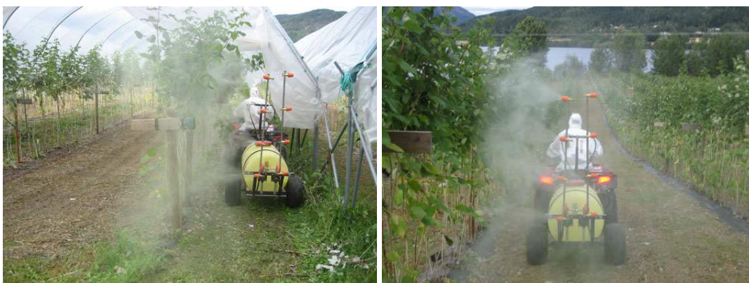
Figure 2. Spraying with ATV and trailed sprayer to the left side only. In the tunnel (left) and in the open field (right). Drift of droplets can be visually seen in the open field situation.
