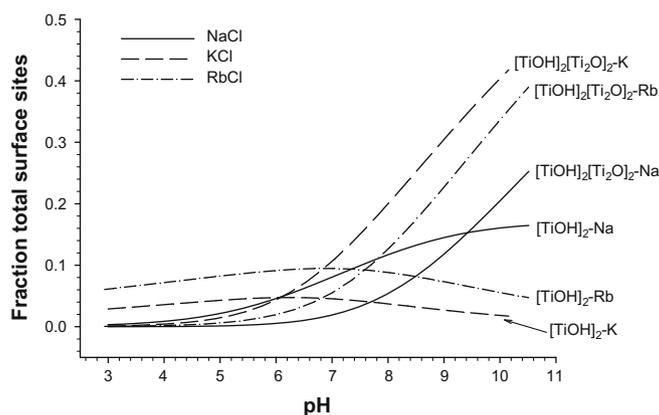
Fig. 6. The distribution of surface species on rutile in solutions comprising electrolyte only at  $I = 0.3 \text{ m}$ . The plots show inner- and outer-sphere electrolyte cation surface species, presented as fractions of the total concentration of surface sites,  $N_s$ , which was fixed at  $20.8 \mu\text{mol/m}^2$ . The anion surface species are omitted for clarity; however, except at low pH conditions the total fraction of anion surface-species is always small.
