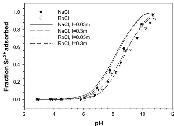
Fig. 5. Adsorption “pH edge” data for the fraction of  $\text{Sr}^{2+}$  adsorbed to the rutile surface relative to total available  $\text{Sr}^{2+}$  in the system, as a function of pH. The symbols represent experimental data at ionic strengths of 0.03 (circles) or 0.3 m (triangles), in NaCl (closed symbols) and RbCl (open symbols) media. All curves represent the CD-MUSIC model best-fits. All model parameter values are defined in the text and are given in Table 1.
