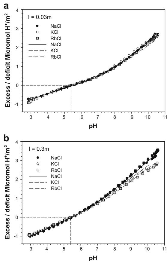
Fig. 2. Titration data showing the effect of electrolyte cation type on the relative proton adsorption/desorption at ionic strengths of 0.03 or 0.3 m. All curves represent the CD–MUSIC model fits. The model parameter values are defined in the text and given in Table 1. The dashed vertical and horizontal lines represent the  $\text{pH}_{\text{znp}}^{\text{c}}$  value and the zero surface charge value, respectively.
