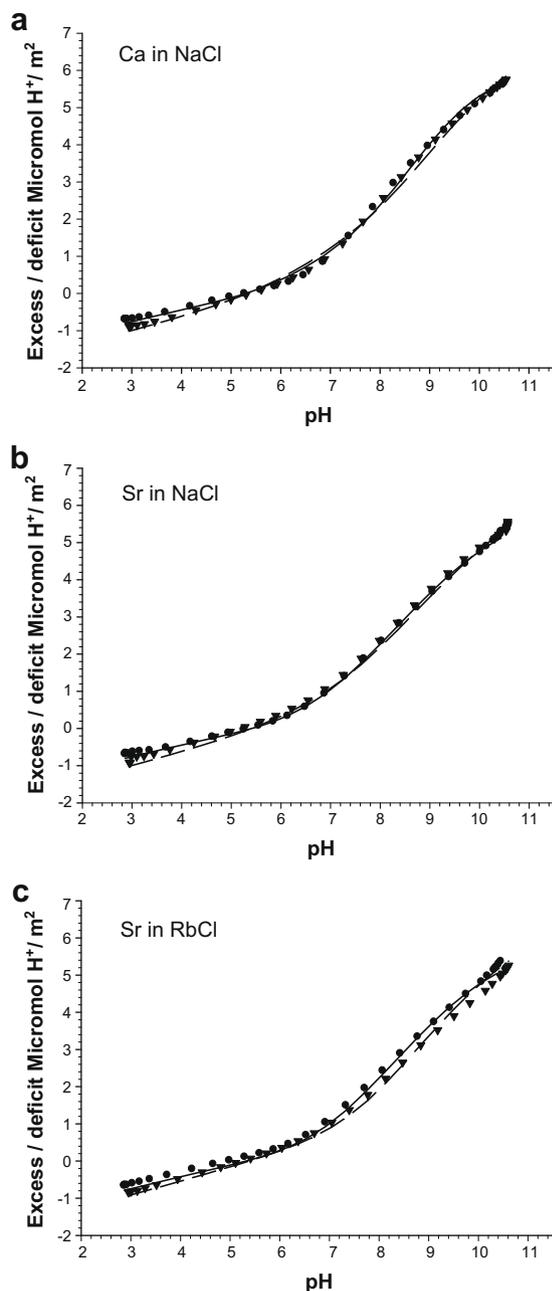
Fig. 4. CD-MUSIC model fits of the relative proton adsorption/desorption and pH titration data for the adsorption of  $\text{Ca}^{2+}$  and  $\text{Sr}^{2+}$  at the rutile surface. All model parameter values are defined in the text and given in Table 1. The symbols represent experimental data at ionic strengths of 0.03 (●) or 0.3 m (▼). The best-fit model curves are shown at 0.03 (solid lines) and 0.3 m (dashed lines).
