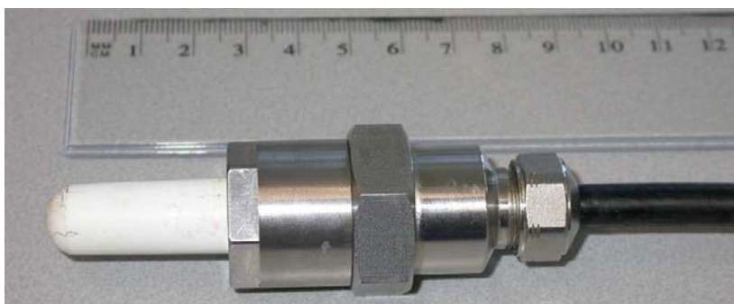
Figure 3-2. Polymer tensiometer with cone-shaped ceramic.
