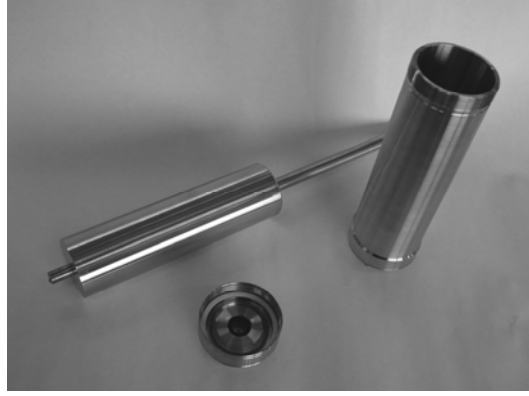
Figure 2. Shearing device with rotating inner cylinder (left) and static outer cylinder (right).
