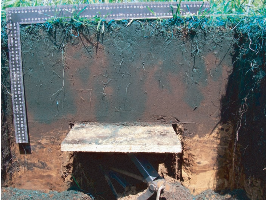
Figure 5.16: Brilliant Blue staining pattern in a soil profile above the seventh row of the metal sampler (see Figure 5.13), at 21 cm distance from the trench side of the instrument. The sampler has been replaced by a plate to support the soil during excavation.
