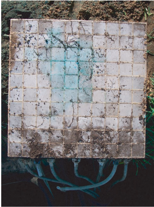
Figure 5.13: The surface of the metal sampler after the Brilliant Blue experiment, with clear dye-staining. The rows of cells discussed in the main text and subsequent figures run from bottom to top. The bottom row was closest to the installation trench. The size of one individual cell is 31.5 \times 31.5 mm.
