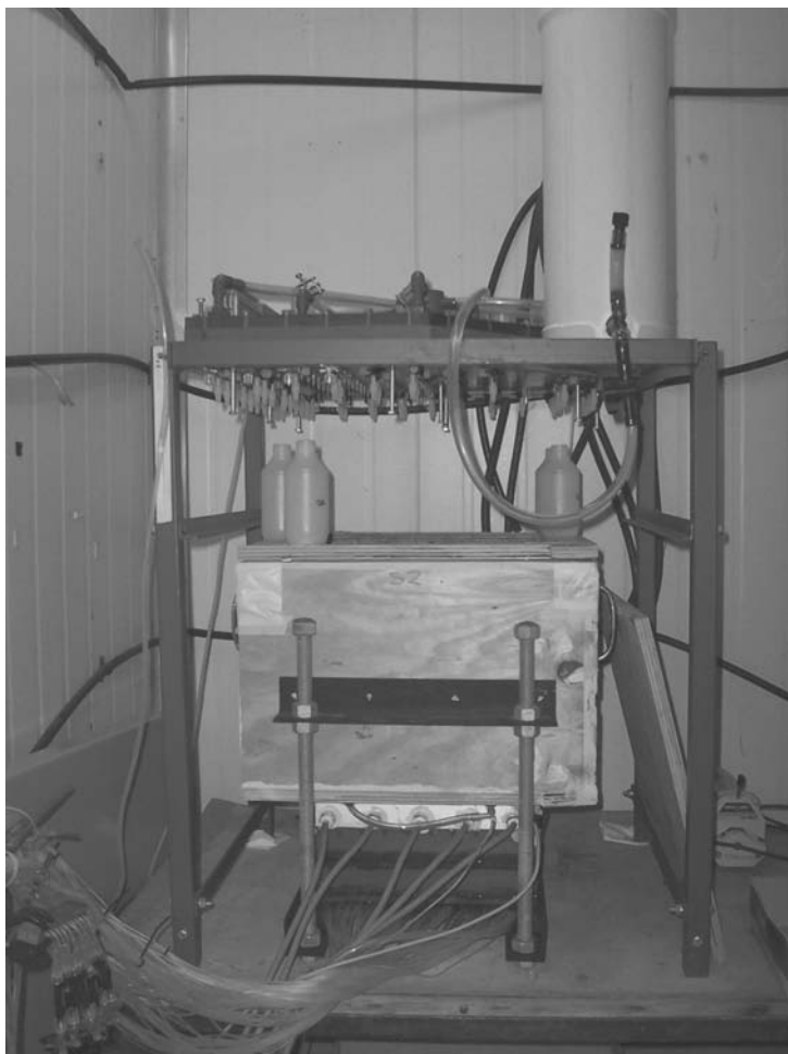
Figure 3.4: The laboratory set-up with the nylon sampler. The multi-compartment sampler is placed on the table, under the soil column in its plywood casing. Above the soil column the rainfall simulator is installed.
