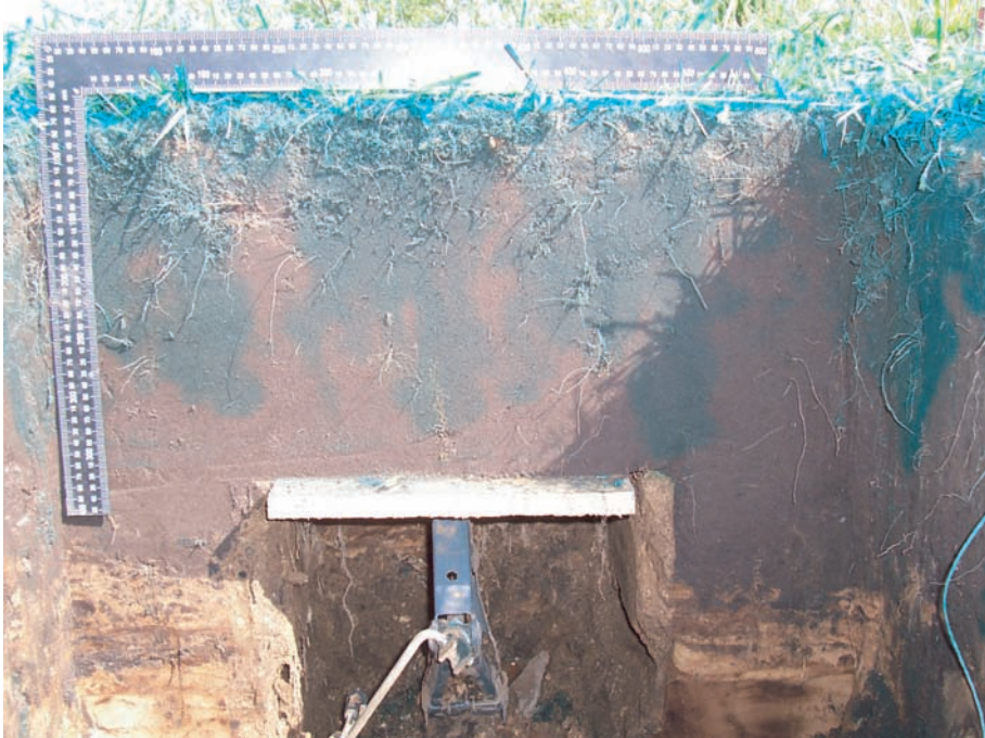
Figure 5.15: Brilliant Blue staining pattern in a soil profile above the third row of the metal sampler (see Figure 5.13), at 8 cm distance from the trench side of the instrument. The sampler has been replaced by a plate to support the soil during excavation. Light-colored soil on either side of the plate is backfilling material around the sampler to minimize the disturbance of the flow pattern.
