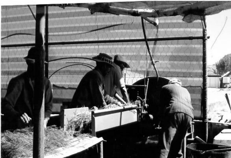
Plate 18. Rooibos bundles are dismantled and put through the cutter
