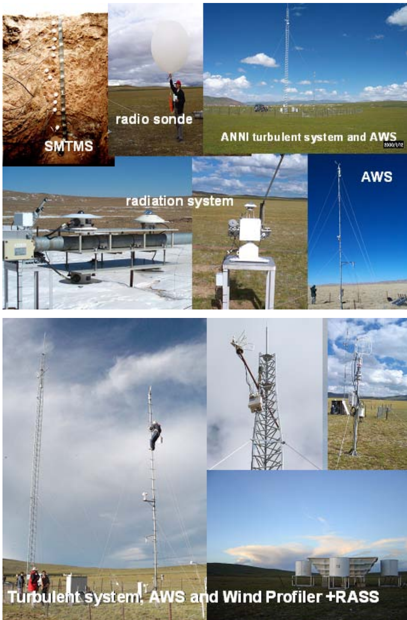
Figure 4.4 Land surface condition and instruments in the stations of the Coordinated Enhanced Observing Period (CEOP) Asia-Australia Monsoon Project on the Tibetan Plateau (CAMP/Tibet).
