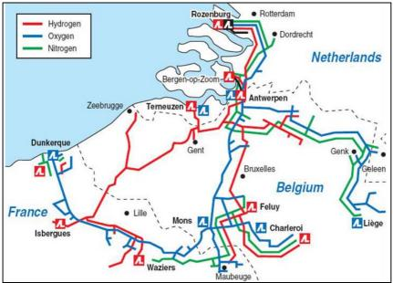
Figure 3 The Air Liquide pipeline network in north-west Europe.<sup>31</sup>
