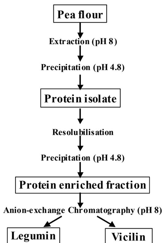
**Figure 1:** Flowchart of legumin and vicilin purification
