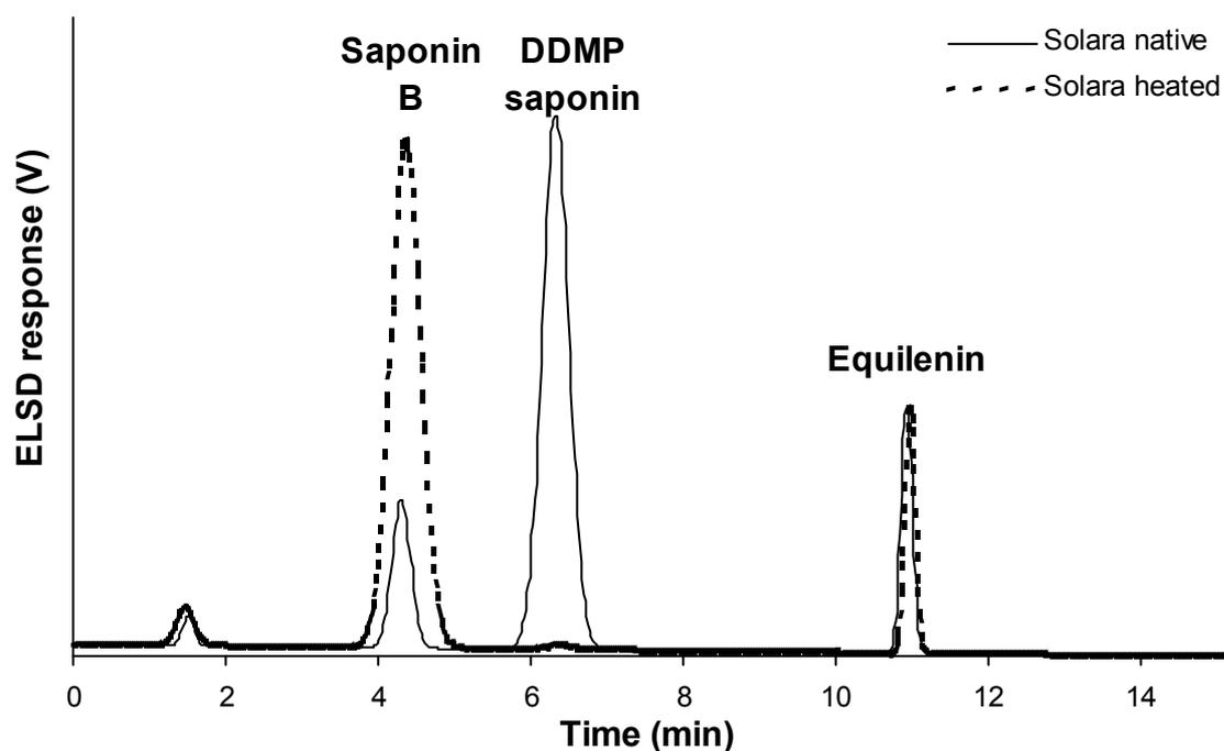
**Figure 2:** Representative RP-HPLC profiles of saponin B, DDMP saponin and the internal standard, equilenin.
