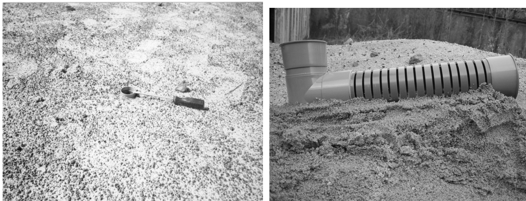
Figure 2) The splash cup (A) and the overland flow detector (B).
