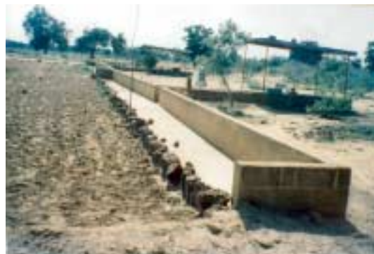
Runoff collection device of the experimental plots at Kirsi village, Burkina Faso
