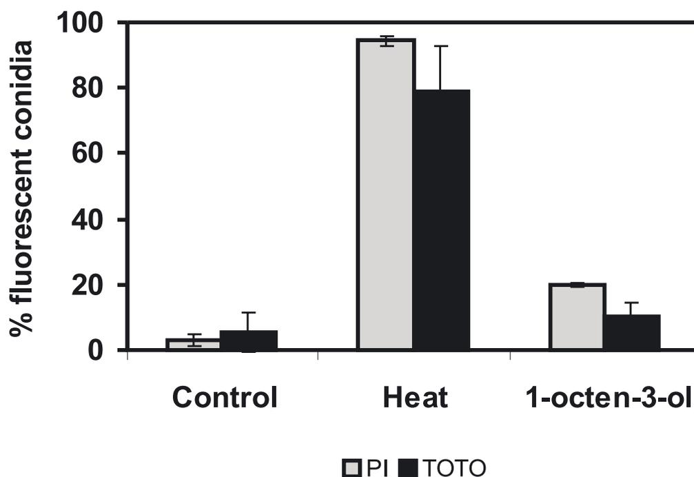
**Fig. 2** Effect of 4 mM 1-octen-3-ol on fluorescent staining of *P. paneum* conidia. Conidia incubated in MEB, heat treated at 90°C for 10 min and exposed to 1-octen-3-ol for 2 h at 25°C were labelled with fluorescent probes. Percentage of fluorescent PI (■) and TOTO (■) labelled conidia, monitored by epifluorescence microscopy.
