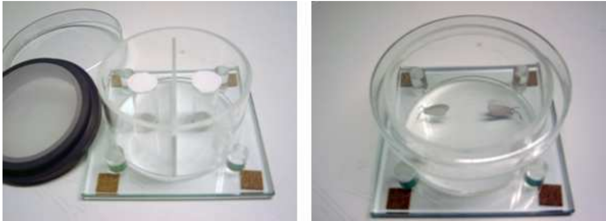
Figure 2: on the left, one can see the olfactometer setup in which filter papers on flasks of glass were used for testing odor combinations I to VII. On the right, the arena for testing the phoretic behavior of T. brassicae in which P. rapae paper models were used for testing phoretic object combinations VIII and IX.
