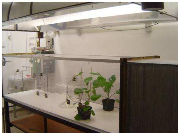
Fig. 11: The wind tunnel set up with two odor sources
