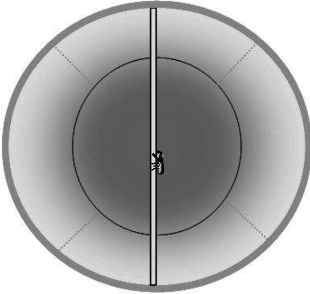
**Figure 2:** Top view of two-choice olfactometer test. The wasp was released in the middle of the two odor fields (decision area).
