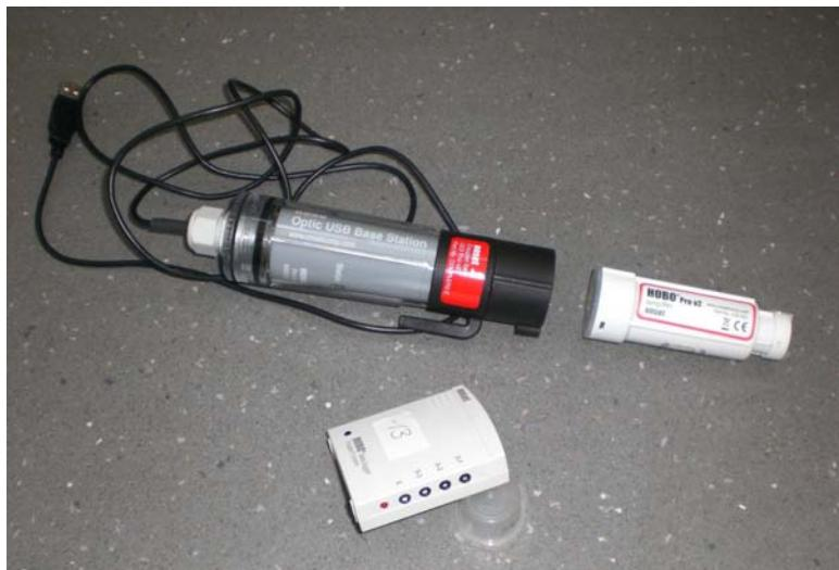
Pic.5. Temperature/RV-logger (above right) with optical base station (above left) and event logger (under).
