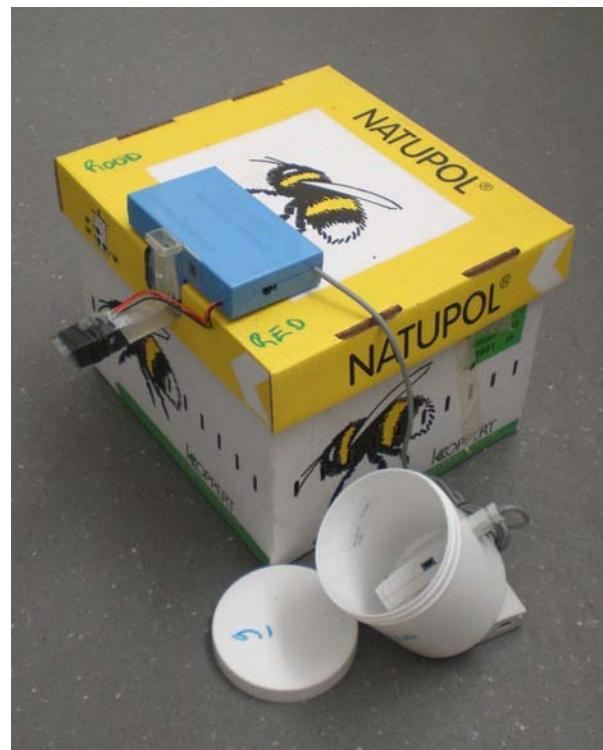
Pic.4. Bumblebee counter with electronic eye (under black tape) and data logger (in white can).
