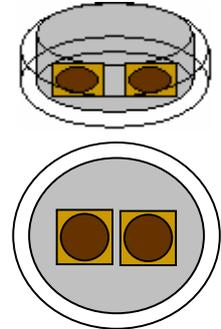
**Figure 6:** Experimental set-up without upper lid. ○ = Outer Petri dish with wet filter paper, ⊙ = Inner Petri dish, ■ = Bark under Petri dish, ● = Bark exposed to weevil.
